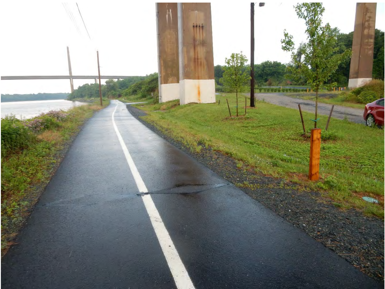
Figure A-11. Combination Passive IR/Inductive Loop Detector in Delaware
